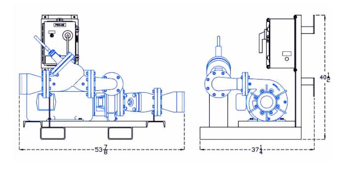
Approximate Shipping Weight (Steel Frame) - 856 LBS, (Aluminum Frame) - 714 LBS Electrical Requirements - Full Load Amps 31.4, Service Factor Amps 36.1, 460/60/3
