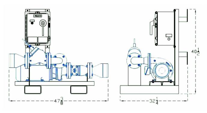
Approximate Shipping Weight (Steel Frame) - 675 LBS, (Aluminum Frame) - 550 LBS Electrical Requirements - Full Load Amps 19.3, Service Factor Amps 24.5, 460/60/3
