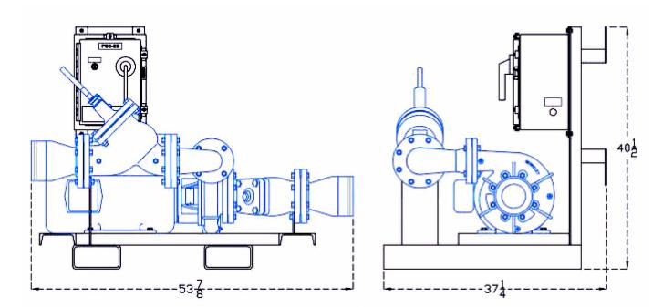
Approximate Shipping Weight (Steel Frame) - 565 LBS, (Aluminum Frame) - 440 LBS Electrical Requirements - Full Load Amps 13.5, Service Factor Amps 15.4, 460/60/3
