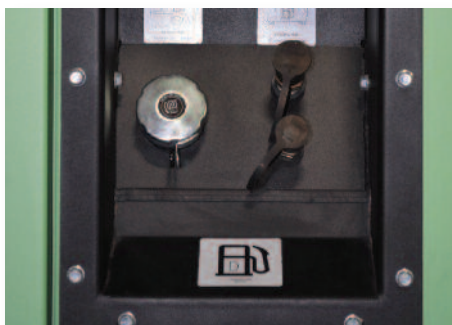
Remote Fuel Panel External fuel fill with remote fuel connections.
